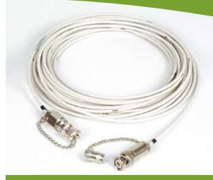
Triaxial BNC (bayonet) connectors are the 2-slot/lug, 1/4-turn locking type. The male connector has a pin insert and is always accompanied by a ferrule with locking slots. It is available only for cable mounting. The female connector has a socket insert and locking lugs that mate with the ferrule. It is available for cable mounting or panel (bulkhead) mounting, with either flange or threaded mounting.
