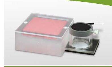
**The Mammographic Accreditation Phantom** is shown with the optional CNMC Model 303 mammographic ion chamber and Model 303ACR chamber holder. Contains: nylon fibrils, simulated microcalcifications and tumor-like masses that mimic the actual
