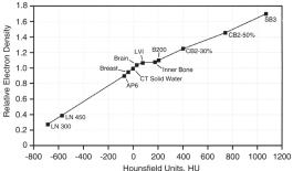
Relationship between relative electron density and CT number (in Hounsfield units, HU) of materials in the Electron Density CT Phantom as measured by GE CT/i scanner.
